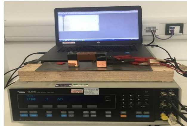
U-shaped sensor is driven using Impedance analyser Solartron 1260
